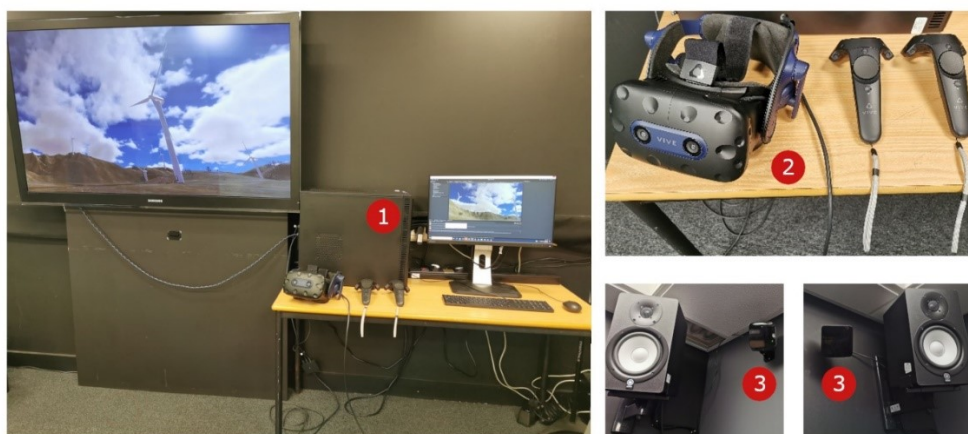
Figure 1: Equipment used to build and test the game. 1) Desktop PC – CPU: Intel® Core™ i7-6700K CPU @ 4.00GHz, RAM: 32 GB RAM, SSD: 1 TB, GPU: Nvidia GTX 1070 8GB. 2) HTC Vive Pro 2 headset and controllers. 3) Wall mounted HTC Vive base station sensors.
