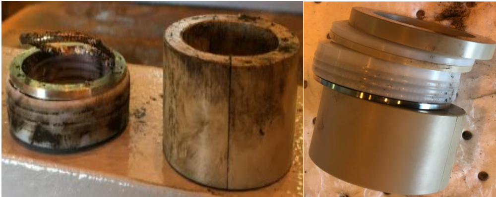
Figure 2 (a) Failed stem packing o the left and new stem packing on the right
