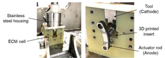
Fig. 4 – ECM setup for insert trial test.
