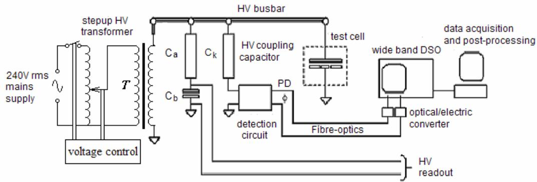
Figure 1 Experimental system showing both HV and detection circuits.
