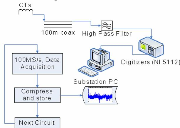
Figure 6 The setup of condition monitoring system in EDF Energy.
