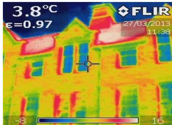
**Figure 4 Solar Gains to SW Roof Surface**
