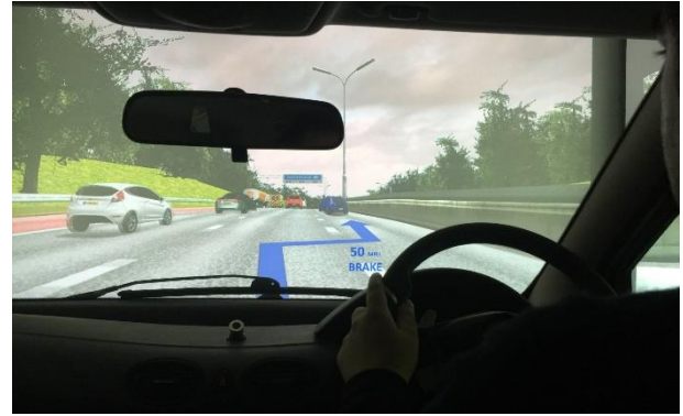
Fig. 2 The Autonomous vehicle (AV) provides visual information through the AR HUD preparing the driver for any collision avoidance manoeuvres [22].
