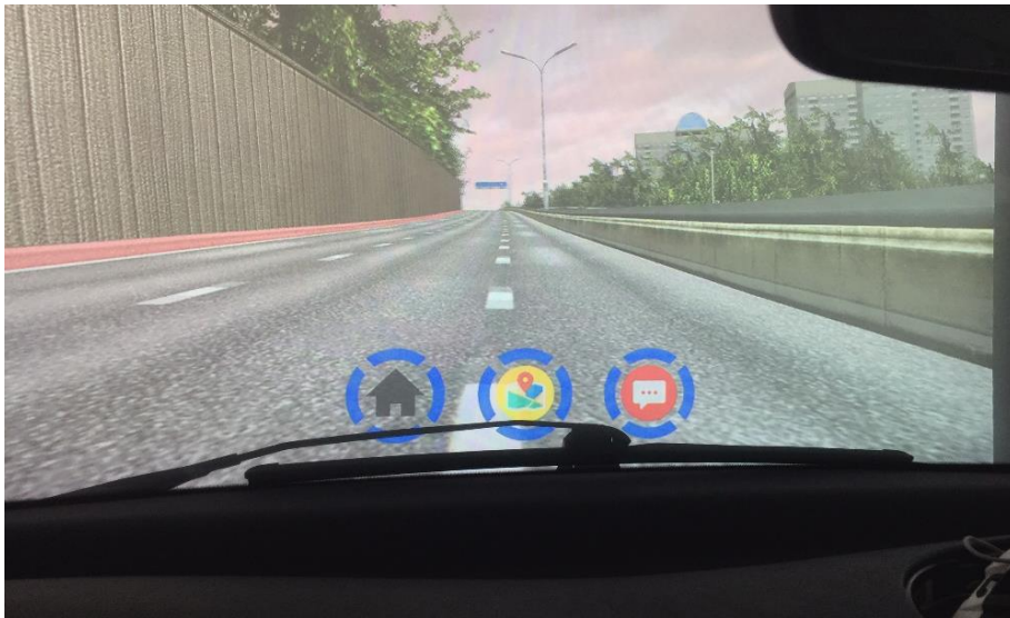
Fig. 3. Simulation Screenshot of the AR HUD and gesture recognition for controlling infotainment sources.
