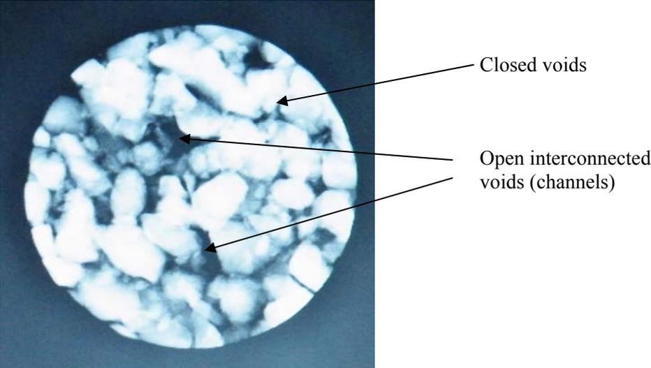
NFC cores analysed show the cores have both closed and open voids. To identify the nominal void size of these NFC cores a capillary rise test was used (see Figures 6, 7 and 8). This section also discusses the relationship between the void size and depth of water ingress, in relation to time. It will also determine the porosity of the NFC cores and the percentage of voids in each core (refer to Figure 9).
