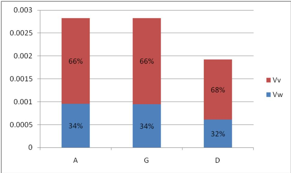
For all the three samples, the porosity level of the NFC cores was 0.66. Everett (1993) indicates the porosity of peat and clay to be more than 0.5 and for stones i.e. granite 0.01. To determine the percentage of the voids refer to Appendix 1.
