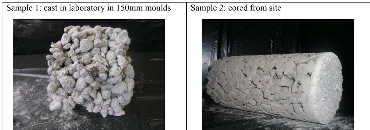
Figure 2 illustrates the difference in the NFC structure of the samples made in laboratory and cored from sites. The laboratory samples were made of river gravel (rounded edges) as coarse aggregate and cores from the site were made of crushed whinstone (sharp edges): the densities of both samples are shown in Table 2
