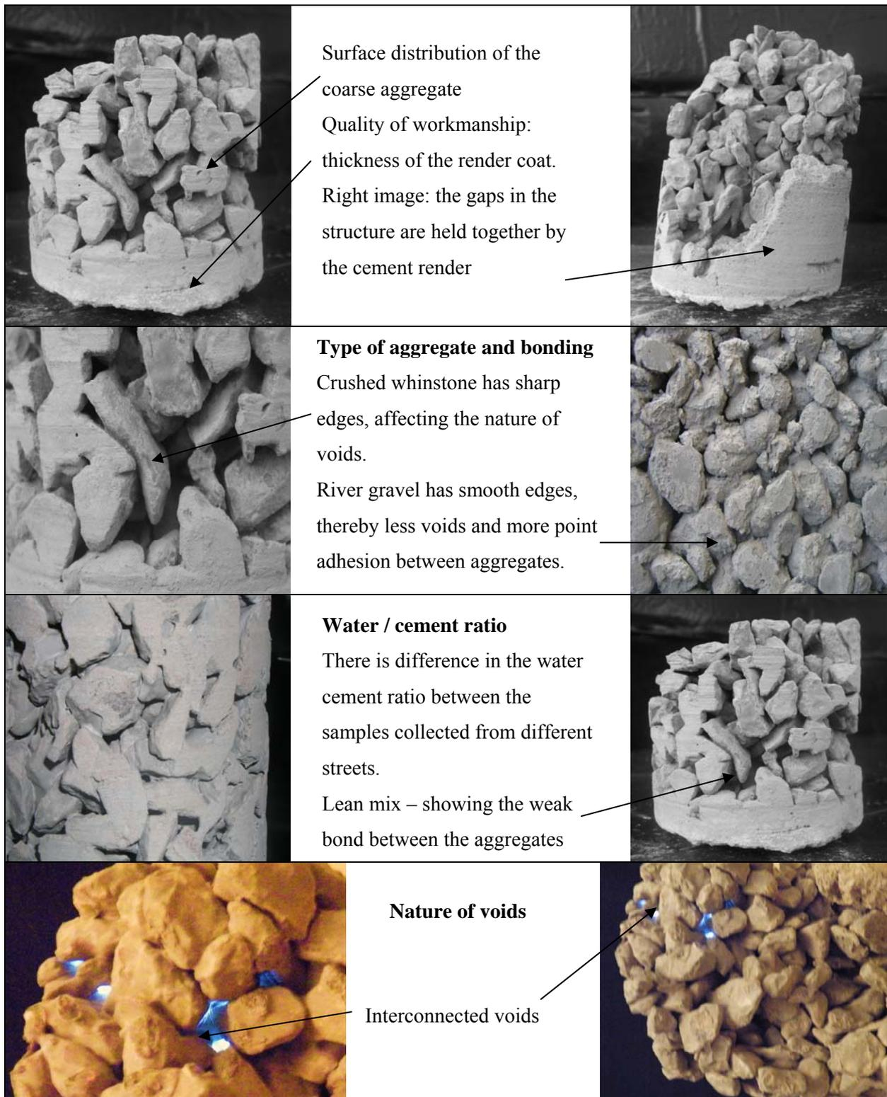
For a clearer picture of the nature of voids in NFC, an x-ray of the section of the core was captured as can be seen in Figure 5.
