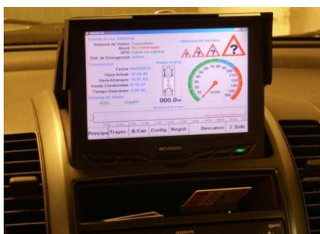
The front-end of the HMI is organized in multiple tabs giving users direct access to the different functionalities. The last four detected traffic signs are displayed on the main HMI screen. In the case of a traffic violation, a warning is emitted in the form of acoustical messages through the vehicle loudspeakers. Finally, drivers can also selectively activate or deactivate some of functionalities. Figure 4 shows a snapshot of the HMI software application.
