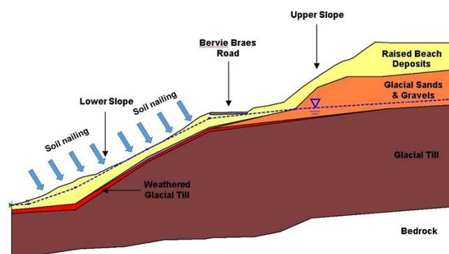
Figure 2. Typical ground profile in the site area
