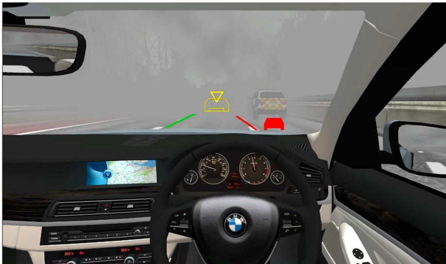
Fig. 1. Previous collision avoidance systems which incorporated AR projection of data through a full-windshield HUD [12].
