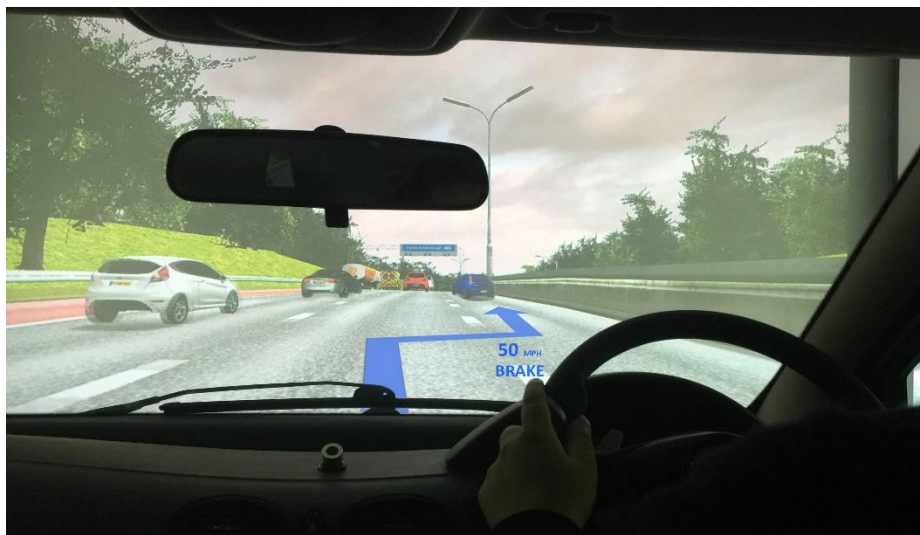
Fig. 4. Suggested manoeuvre and speed by AR/AI HUD in a driving simulation environment.
