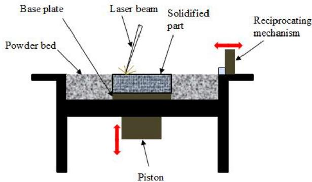
**Figure 1.** Basic components of a typical SLM machine
