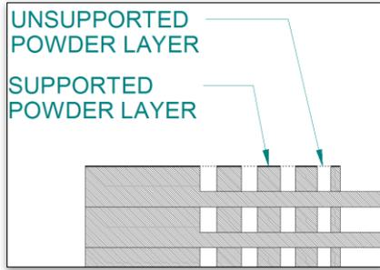
Figure 11. Supported and unsupported areas on the discs
