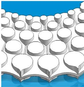
Figure 12. Single disc view for the new design
