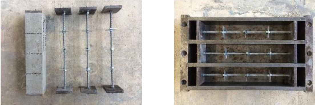
Figure 2: Designed moulds for plastic shrinkage tests.
