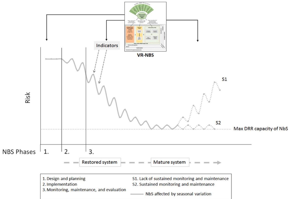
**Fig. 4.** Risk levels throughout time (denoted by NBS phases) of an idealized NBS that relies on organic elements to reduce risk. Risk reduction can thus fluctuate seasonally. The VR-NBS framework can be applied throughout NBS phases to assess vulnerability and risk and contribute to successful NBS design and long-term monitoring and maintenance to achieve sustained and maximum disaster risk reduction capacity. Indicators from the framework can be applied to capture changes in seasonality.
