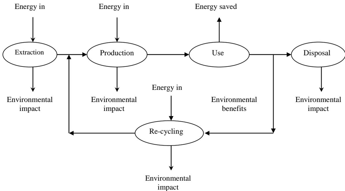
Figure 1: Typical life cycle of building products
