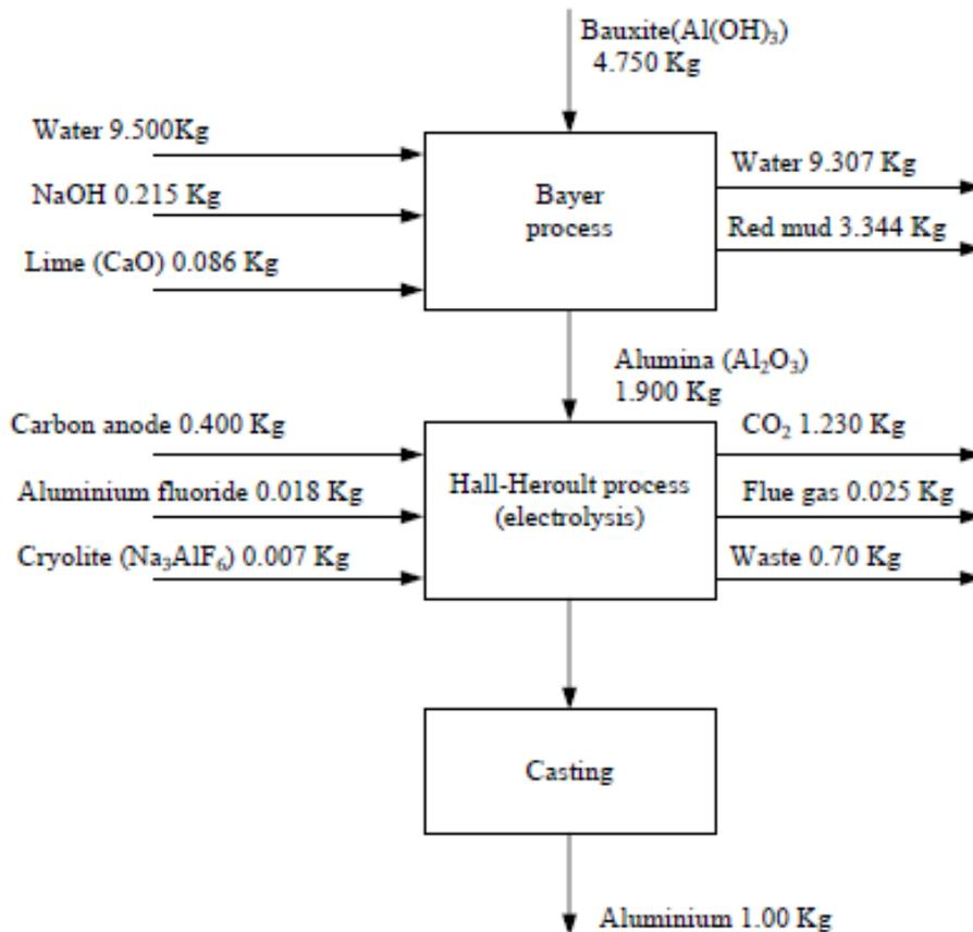
Figure 6: Primary aluminium production from raw material
