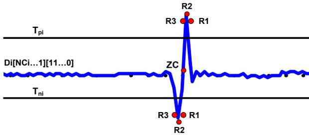
Fig. 7. Finding modulus maxima from  $D_i(n)$ .
