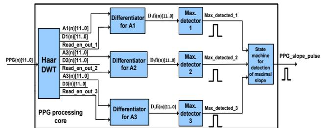
Fig. 9. Internal structure of PPG slope detection core.
