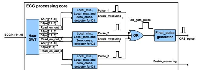
Fig. 5. Internal structure of ECG processing core.
