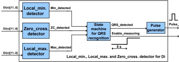
Fig. 6. QRS detection from  $D_i(n)$  - structure.
