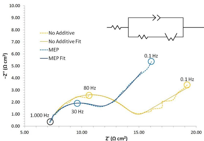
**Figure 4.** EIS data obtained at  $E_{1/3}$  in the solution containing 50 mM  $\text{ZnBr}_2$ , 0.5 M  $\text{KNO}_3$  with no additive (orange) and with 16.67 mM MEP (blue) at a GC electrode.  $T = 295 \text{ K}$ . Inset shows equivalent circuit used for fitting the data.
