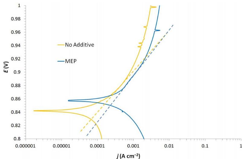
**Figure 5.** Tafel slopes (dashed lines) obtained from potentiodynamic curves in a solution containing 50 mM ZnBr<sub>2</sub>, 0.5 M KNO<sub>3</sub> with no additive (orange) and with 16.67 mM MEP (blue).
