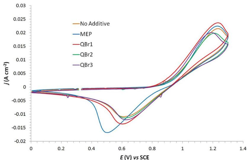
**Figure 3.** Cyclic voltammograms at a glassy carbon electrode in 50 mM  $\text{ZnBr}_2$ , 0.5 M  $\text{KNO}_3$  with 16.67 mM of either MEP, QBr1, QBr2 or QBr3. Scan rate of  $50 \text{ mV s}^{-1}$ .  $T = 295 \text{ K}$ .
