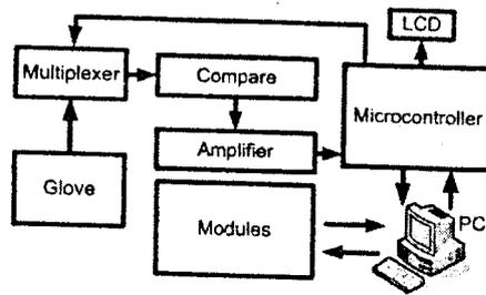
Figure 3. The hardware structure of the system
