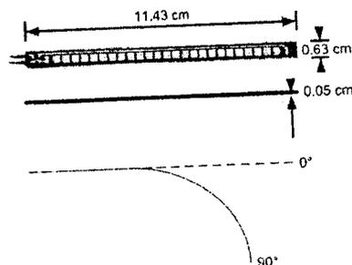
Figure 2. The structure of flex sensor
