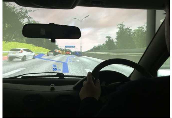
Fig. 5. Screenshot of HUD prototype testing in the Virtual Reality Driving Simulator Laboratory.
