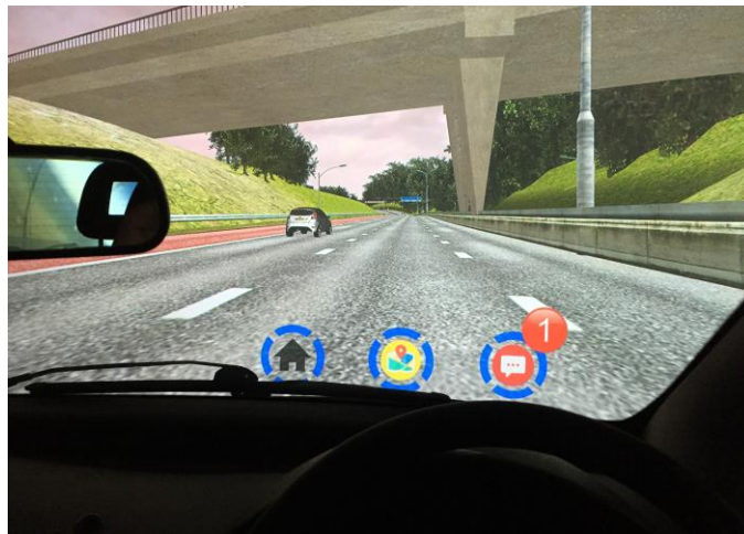
Fig. 3. Final HUD interface with 3 icons in action during simulation.
