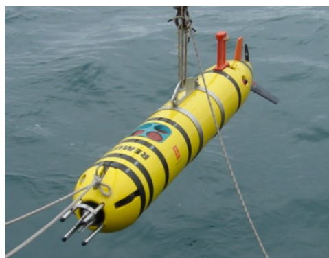
Figure 6. The Scottish Marine Robotic Facility –AUV Remus 600
