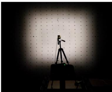
Fig. 12. Footprint of the RDTIRO-LED system at 1 m distance from the centre of the target plane.
