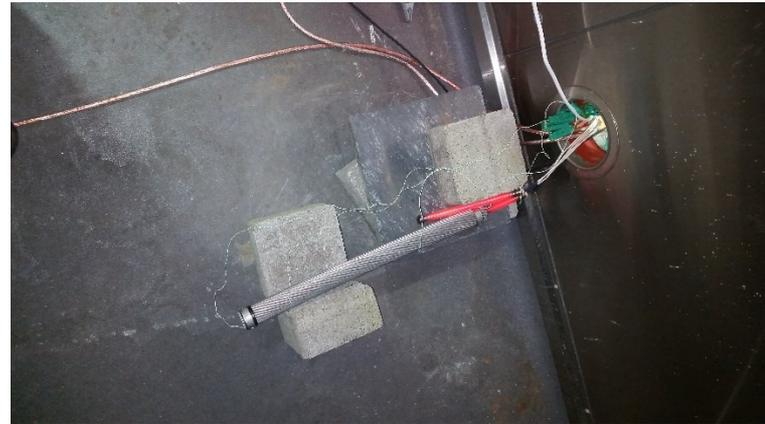
Fig 1- Calibrating the cartridge heater feedback thermocouple
