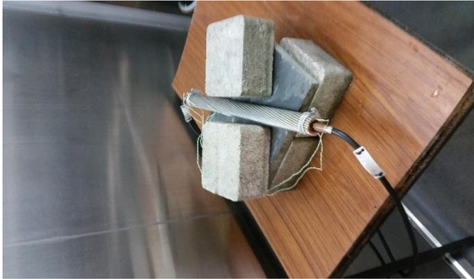
Fig 3- Pre-test setup; AAAC cable, stranded Araucaria conductor
