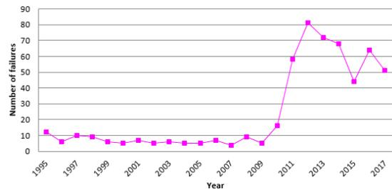
Fig. 2. Number of cable failures 1995 -2017 (33kV)
