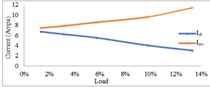
Fig. 6 Loop currents for increasing load for 1 shorted turn in primary winding
