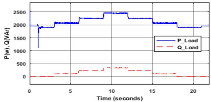
Fig. 14. Increasing of load active and reactive power
