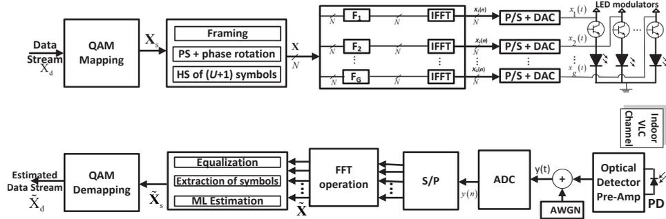
Figure 1: Block diagram illustrating the architecture of the pilot-assisted O-OFDM system with multiple LED groups. PS: pilot symbol, HS: Hermitian symmetry, P/S: Parallel-to-serial, S/P: serial-to-parallel, ADC: analog-to-digital converter, ML: Maximum likelihood
