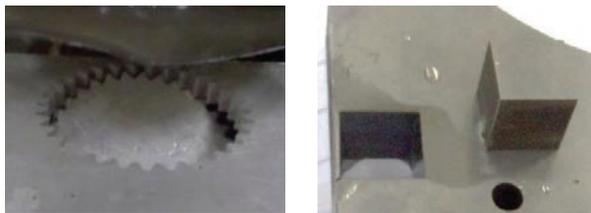
Fig. 1. (a) Gear profile with Al alloy (b) Square profile with steel
