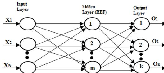
**Figure 5** The basic structure of RBF network [85]
