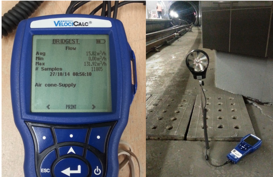
Figure 5: The portable air velocity meter with the attached rotating vane
