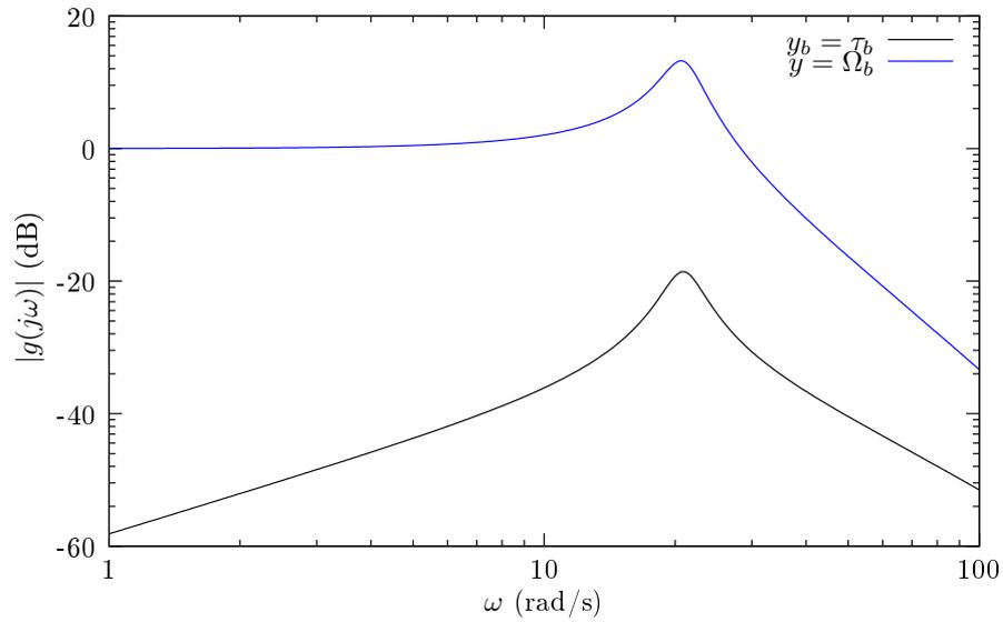
Figure S2: Frequency response for the Quanser experiment. The numerical values of Table S1 combined with the bond graph of Figure S1 yield the frequency response of  $y = \Omega_b$  and  $y_b = \tau_b$ , measured in rad/s and N-m respectively, to the equivalent system input  $u_0$ , measured in rad/s; the resonant peak corresponds to the flexure natural frequency of about 20 rad/s.
