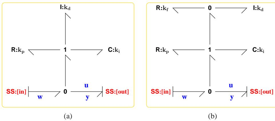
Figure 11: PID Control. (a) Pure PID.  $\mathbf{R}:k_p$ ,  $\mathbf{C}:k_i$ , and  $\mathbf{I}:k_d$  give the proportional, integral and derivative terms, respectively;  $\mathbf{I}:k_d$  has *derivative* causality. (b) Filtered PID.  $\mathbf{R}:k_f$  and the associated  $\mathbf{1}$  junction give a lowpass filtering effect on the derivative action;  $\mathbf{I}:k_d$  now has *integral* causality.
